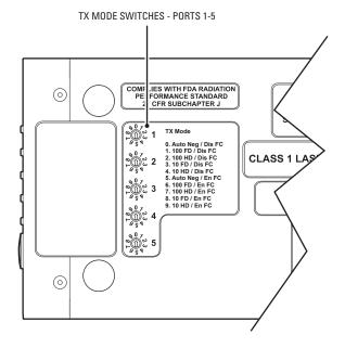
Figure 4. TX Mode Switches for 10BASE-T/100BASE-TX Ports 1-5
